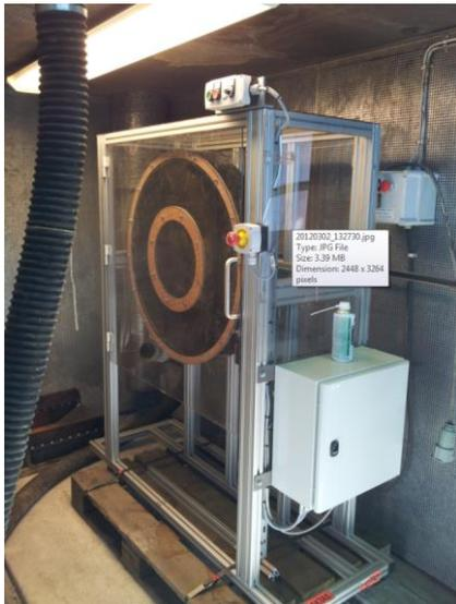
*SSAB's Drum Wear Test consists of an  $\varnothing 800 \times 100$  mm steel drum, where up to 34 samples are placed in a holder, assembled along the inside of the drum and tested under the same conditions.*
