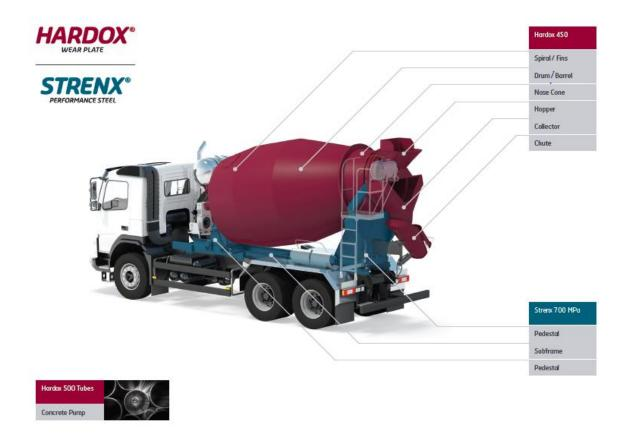
Our comprehensive offering to concrete equipment manufacturers includes Hardox wear plates, sheets and tubes, Strenx high-strength structural steels, as well as tailored solutions on design, product development and processing support available from SSAB SHAPE.
