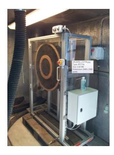
SSAB's Drum Wear Test consists of an  $\emptyset 800x100mm$  steel drum, where up to 34 samples are placed in a holder, assembled along the inside of the drum and tested under the same conditions.
