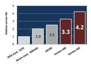
Results from SSAB's Drum Wear Test show that Hardox 450 wear plate enables 4.2 times longer relative service life compared to mild steel S235.
