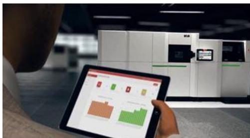
The EOS M 300-4 is equipped with software solutions for all AM process steps – from the preparation of CAD design data and the build job to quality control. (Source: EOS).
